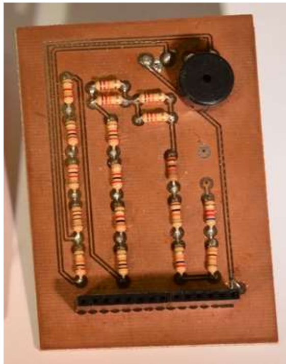
PCB with copper exposed, no solder mask or silkscreen.
